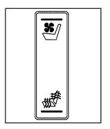
Your vehicle may have heated and ventilated front seats. The buttons are located on the climate control panel.
